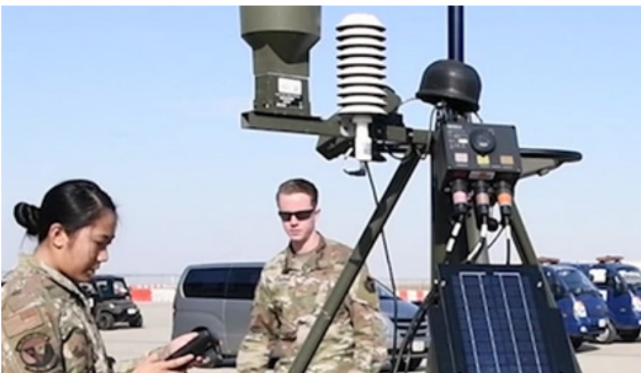
The 607th Weather Squadron setting up a tactical meteorological observing system used to support mission operations. (Department of the Air Force photo by American Forces Network Humphreys)
